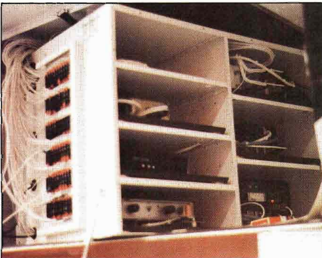
Electronics systems controls from the cockpit are interfaced to the hardware rack in the rear luggage compartment on terminal strips.
